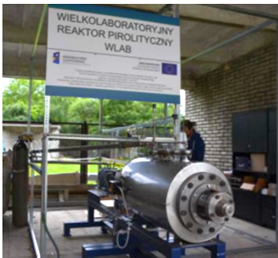
WLAB: large-scale periodically operated pyrolytic reactor
